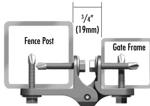
**NOTE:** Kwik-Fit hinges are intended for post mounting only. For mounting to walls where there is no room for a fence post, use D&D's "Multi-Adjust" MFA model.
